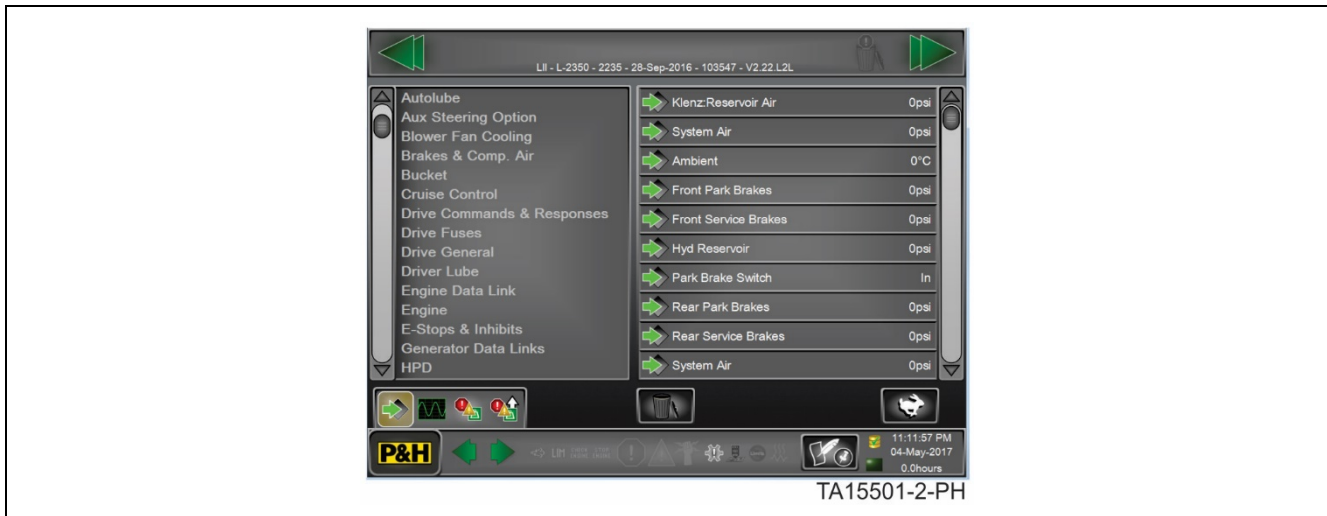
Figure 6. LINCS II channel selection screen (typical screen)
